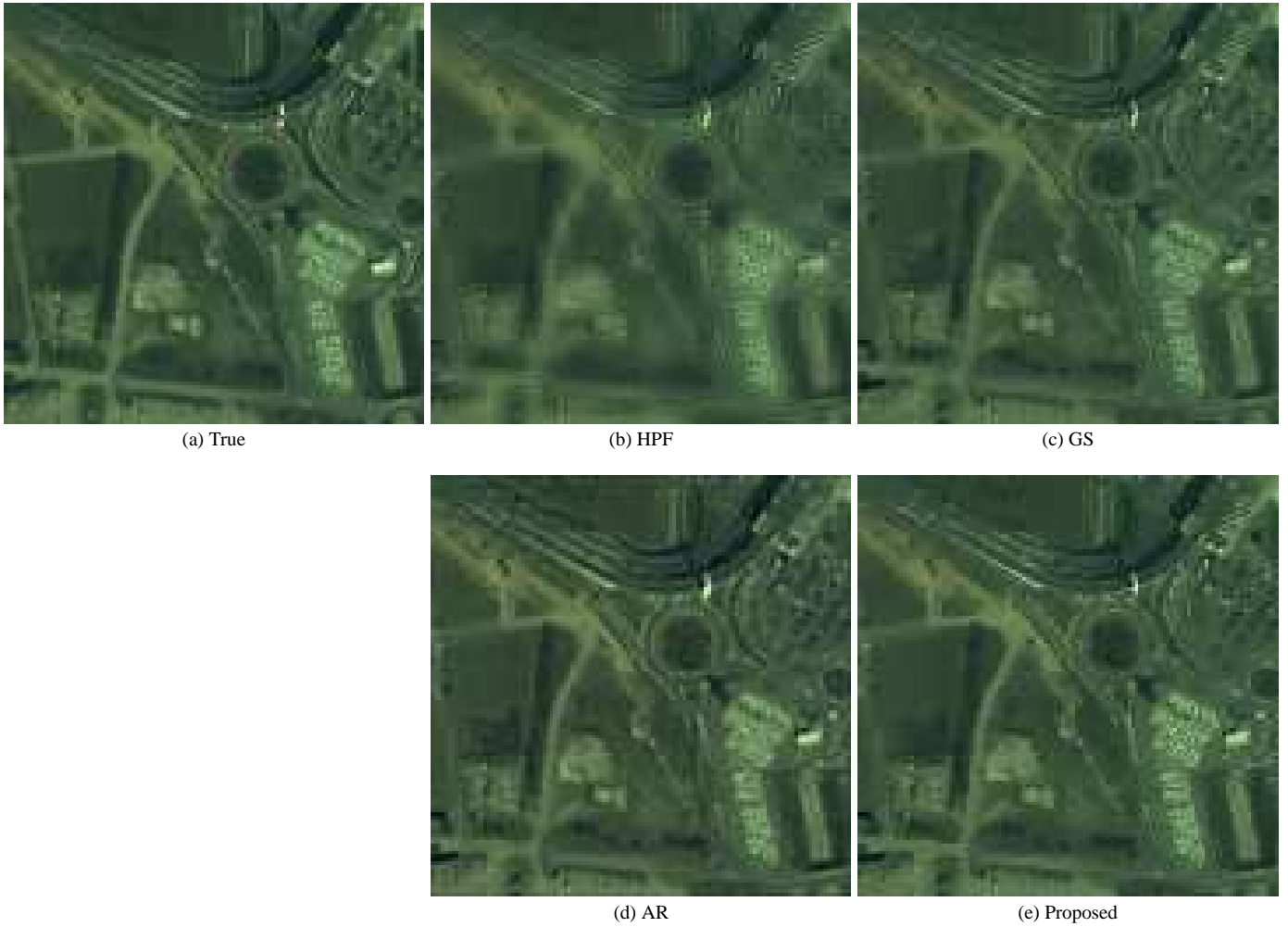
Fig. 5. (a) 128 \times 128 pixels true MS color composite at 2.4 \text{ m} \times 2.4 \text{ m} spatial resolution (3, 2, and 1 color composite), (b) HPF fused MS ( 2.4 \text{ m} \times 2.4 \text{ m} ), (c) fusion using Gram-Schmidt (GS) method ( 2.4 \text{ m} \times 2.4 \text{ m} ), (d) Homogeneous AR model based approach ( 2.4 \text{ m} \times 2.4 \text{ m} ), (e) Fusion using the estimated IGMRF parameters from the high resolution Pan image.
