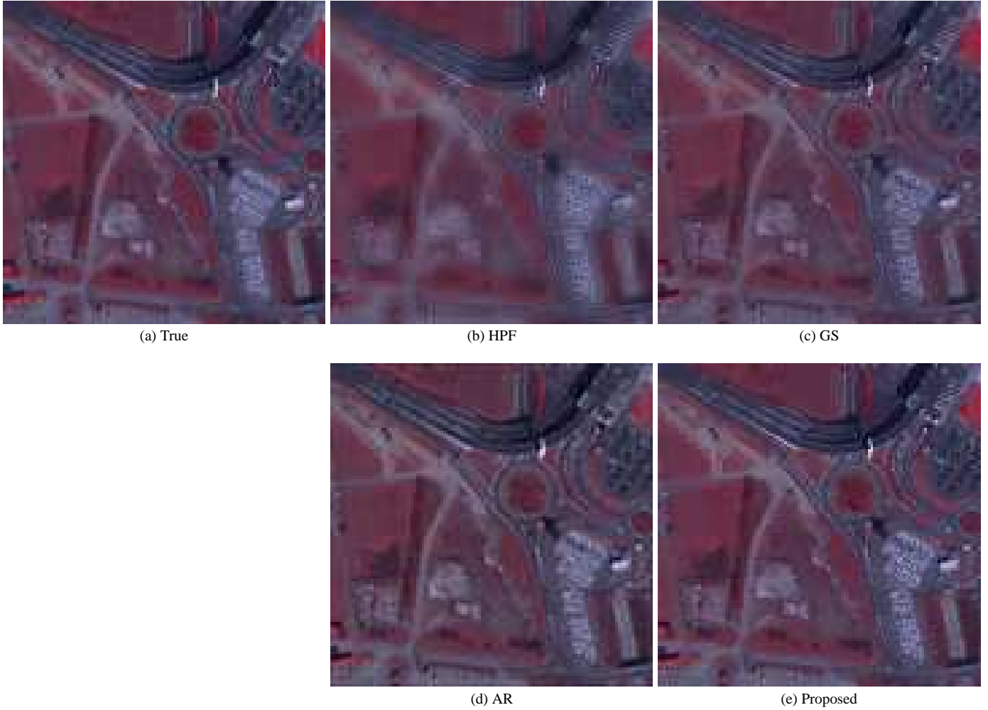
Fig. 4. Fusion results of degraded MS bands 4, 3, and 2 color composite (a) 128 \times 128 pixels true MS color composite at 2.4 \text{ m} \times 2.4 \text{ m} spatial resolution, (b) HPF fused MS ( 2.4 \text{ m} \times 2.4 \text{ m} ), (c) fusion using Gram-Schmidt (GS) method ( 2.4 \text{ m} \times 2.4 \text{ m} ), (d) Homogeneous AR model based approach ( 2.4 \text{ m} \times 2.4 \text{ m} ), (e) Fusion using the estimated IGMRF parameters from the high resolution Pan image.
