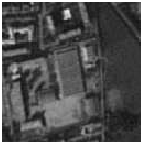
Fig. 14. Image deconvolved with quadratic regularization (SNR=19.5 dB)
